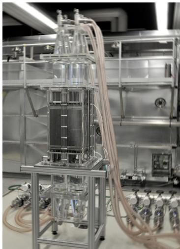
The FA-dummies are encased in an acrylic glass housing and can be connected to the "Zittau Flow Tray". Possible configurations for the investigation of the cross mixing are 2x2 or 1x4. The measurements are identical with the single FA-dummy.
