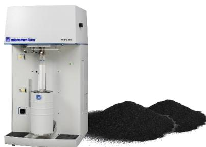
BET surface measured with Micromeritics 3Flex surface analyzer
